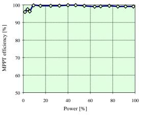
Figure 4. MPPT efficiency of OKE4 [Source: ECN, May 1996]
