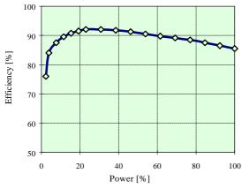
Figure 3. Efficiency of OKE4
