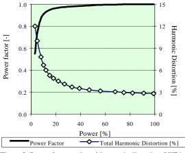
Figure 2. Power factor and total harmonic distortion OKE4
