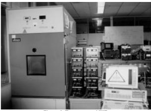
Figure 5. Test set up at NKF. On the left the oven with 10 inverters inside, in the middle 10 PV simulators and on the right the monitoring computer.
